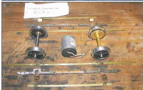
9. Above, left: Bodywork painted and controllers ready for fitting. 10. Above: More detail bits for completion of the body; bumpers, resistance boxes, handbrakes and headlights. 11. Left: Now to the truck. The sideframes are laser cut from mild steel which I have made to a 7ft. wheelbase. (they can be cut in the middle and lengthened/shortened to suit a particular model). All other parts are fabricated from brass, the wheels are from "Slaters" and gear wheels are specially cut for me, ratio of 1 to 5 for 33in. and 1 to 4 for smaller sizes. 12. Below: Truck assembled and motor fitted. The "can" motors are recycled from old video and DVD players! 13. Bottom: Body attached to the truck (as yet unpainted) and just needs a trolley pole and other final details.
